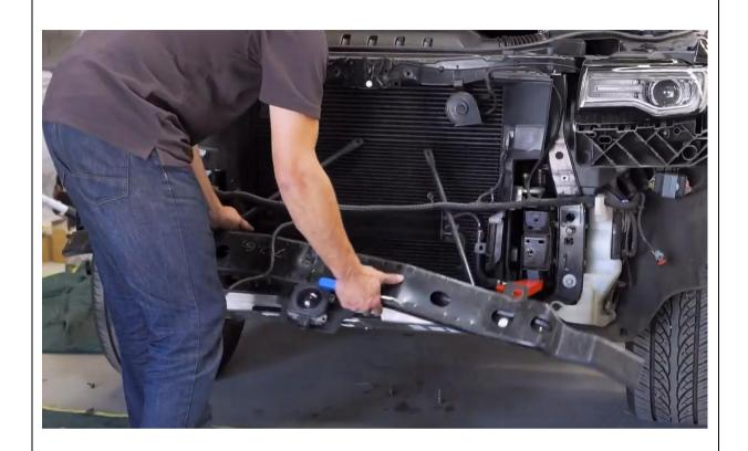
19. Remove 2x screws with 13mm tool holding round support bars from top of bonnet support then remove entire reinforcement bar.
