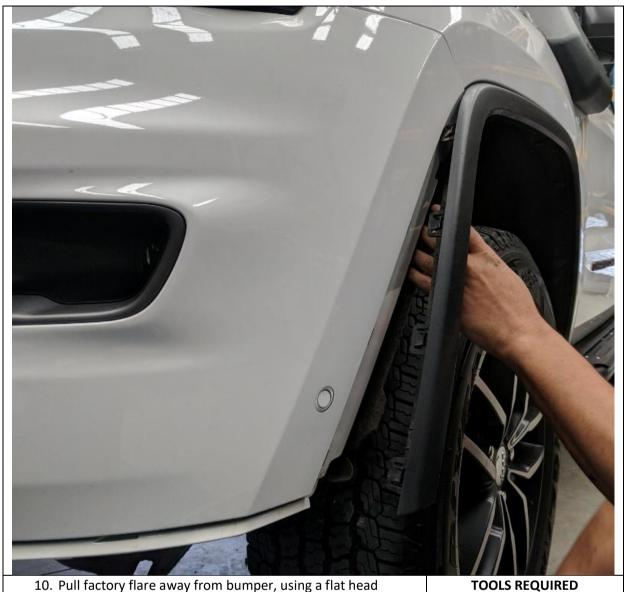
10. Pull factory flare away from bumper, using a flat head screwdriver release at least 2 of the push in clips on top edge being careful not to break them as you pull the flare away from the body.
