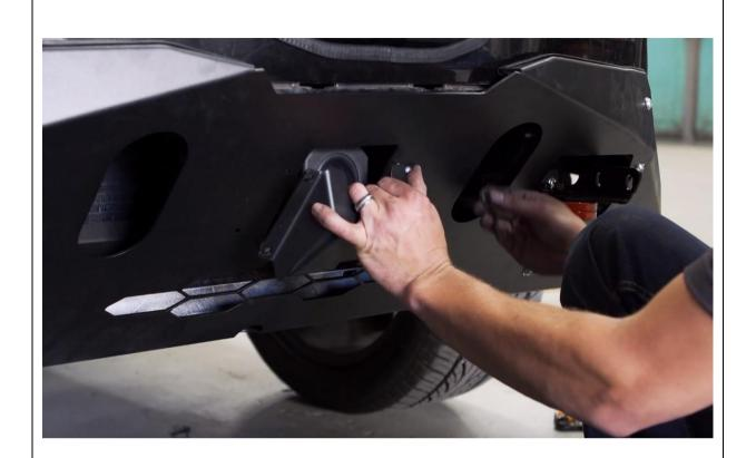
36. Secure ACC cover to main plate with M6 x 16 button head cap screws washers and flange nuts
